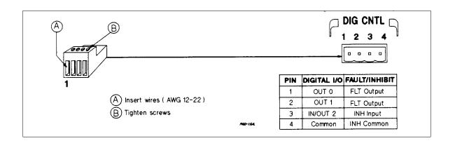
Figure D-1. Digital Port Connector
